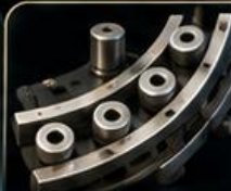
Cam Track (guides movement of punches)
